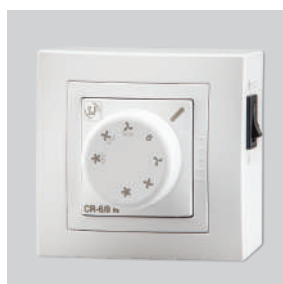
CR-6/9 N 2 Power remote selector and 3 speed fitted with the fan to control up to 5 units in series of the A/H models (ambient and hot air). LxWxH (mm): 88x47x88
